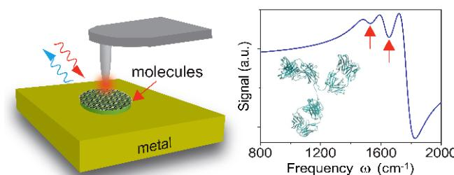
Figure 1. Left panel: schematic of proposed AGP nanoresonator for sensing, namely, graphene nanodisk above a metallic substrate separated by a thin molecular layer, probed by a scattering-type scanning near-field optical tip. Right panel: simulated near-field spectrum of an AGP nanoresonator with a protein layer (sketch of the protein molecule is shown in the inset) in the spacer. The arrows show two vibrational bands of the protein.
