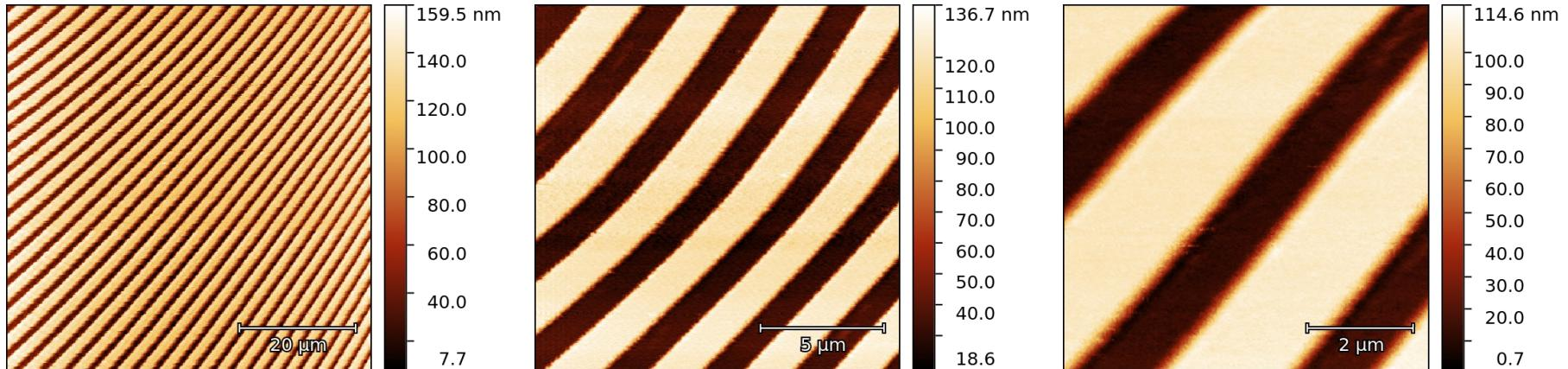
Sample measurement by Akiyama probe (TGZ2 reference grid, nominal period 3  $\mu\text{m}$ , nominal height 110 nm).
